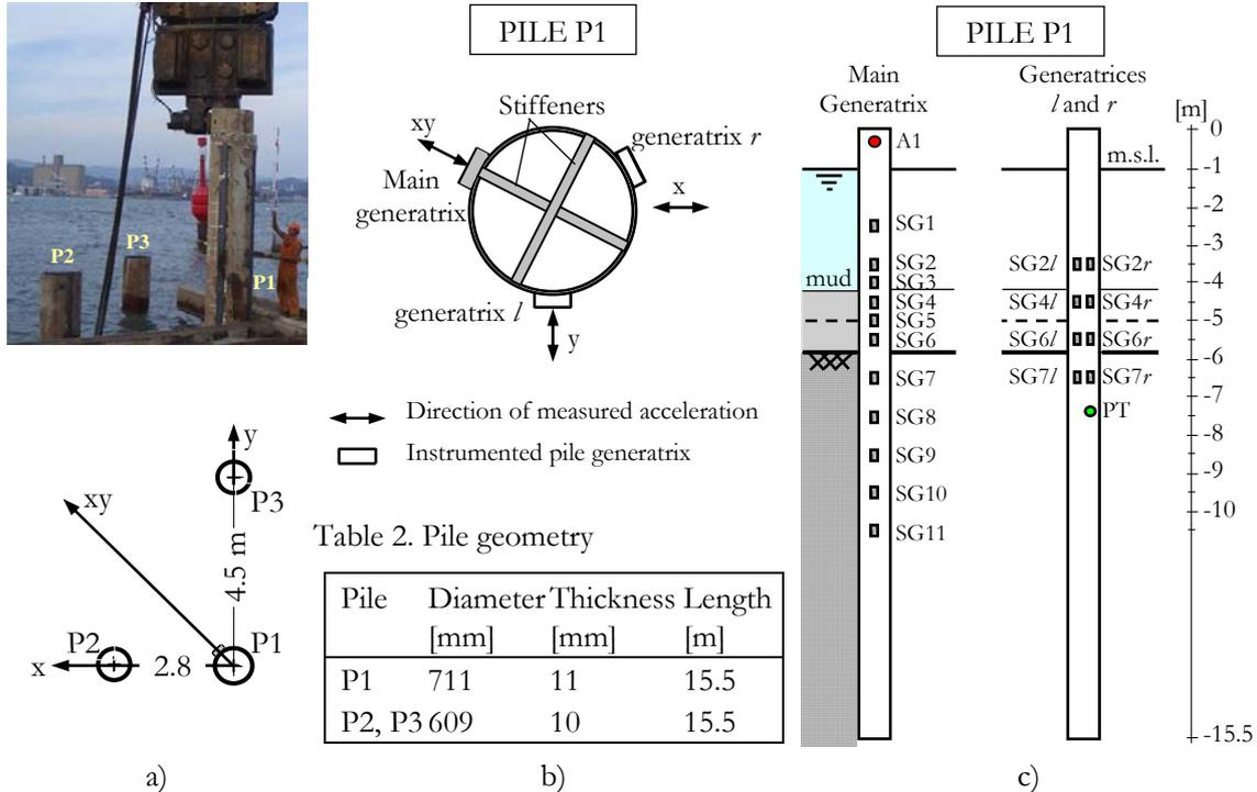
Figure 2. a) Test field; b) Pile P1 plan view and geometric characteristics of the piles; c) pile P1 instrumentation
