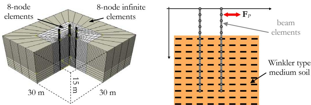
Figure 4. 3-D ABAQUS model on the left and model proposed by Dezi et al. (2009) on the right
