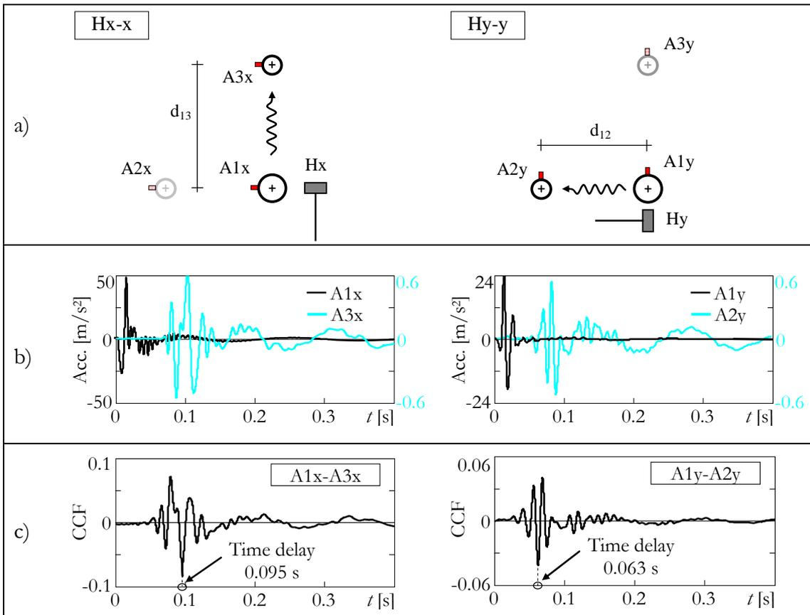
Figure 6. a) Test configurations; b) Time histories of acceleration on source and receiver piles; and c) Cross-Correlation Functions
