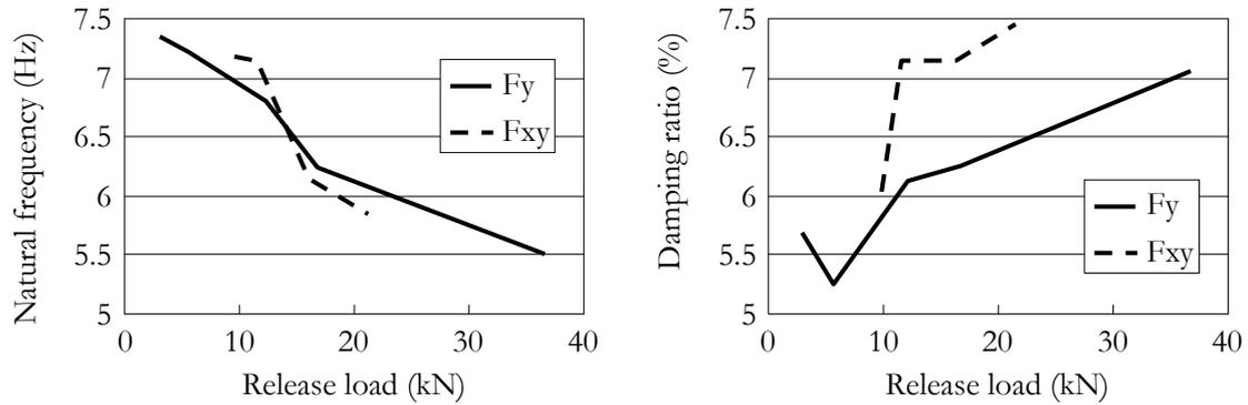
Figure 7. Natural frequency vs load release and damping ratio vs load release
