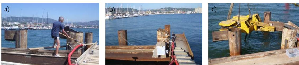
Figure 3. a) Impact load test; b) free vibration test; c) forced vibration test
