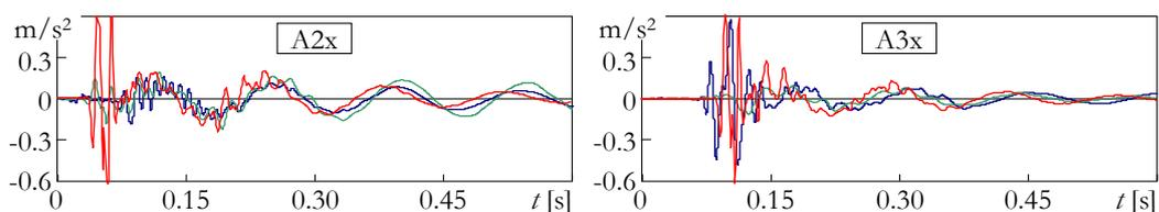
Figure 10. Time histories of accelerations on the receiver piles
