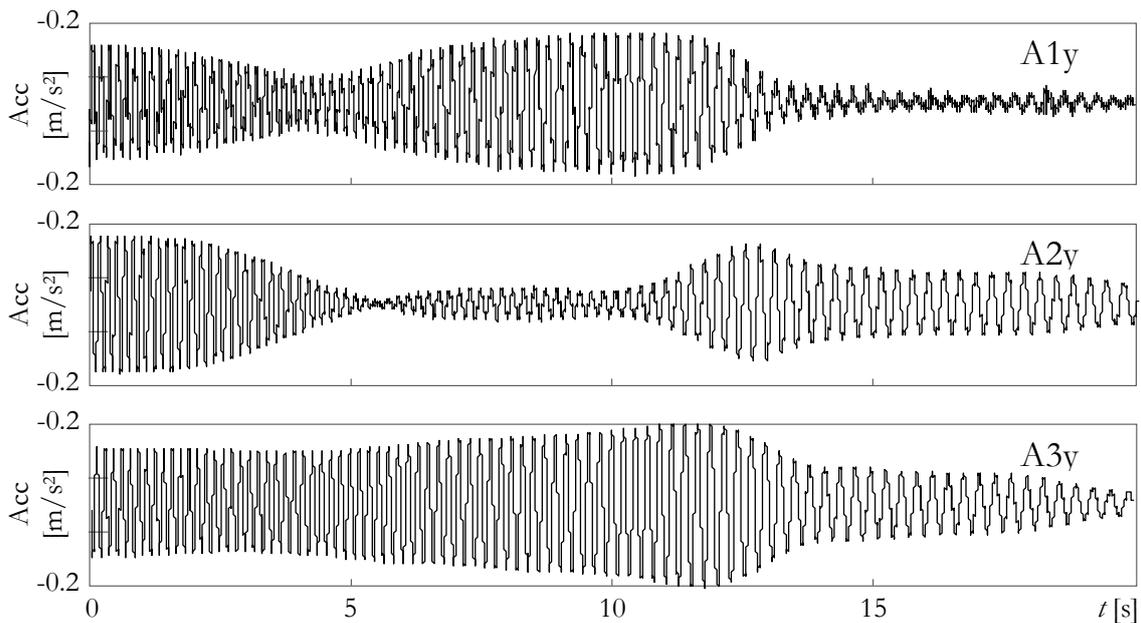
Figure 8. VAxy-y-ee.sweep test : accelerometer signals
